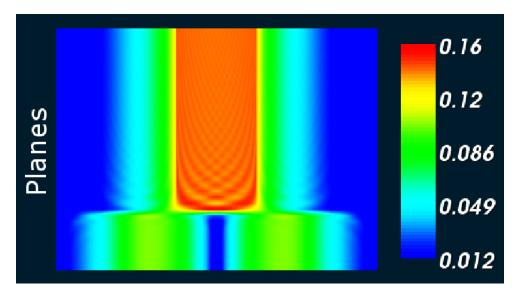
Changing the band offsets creates particle-hole asymmetry in the DOS.
