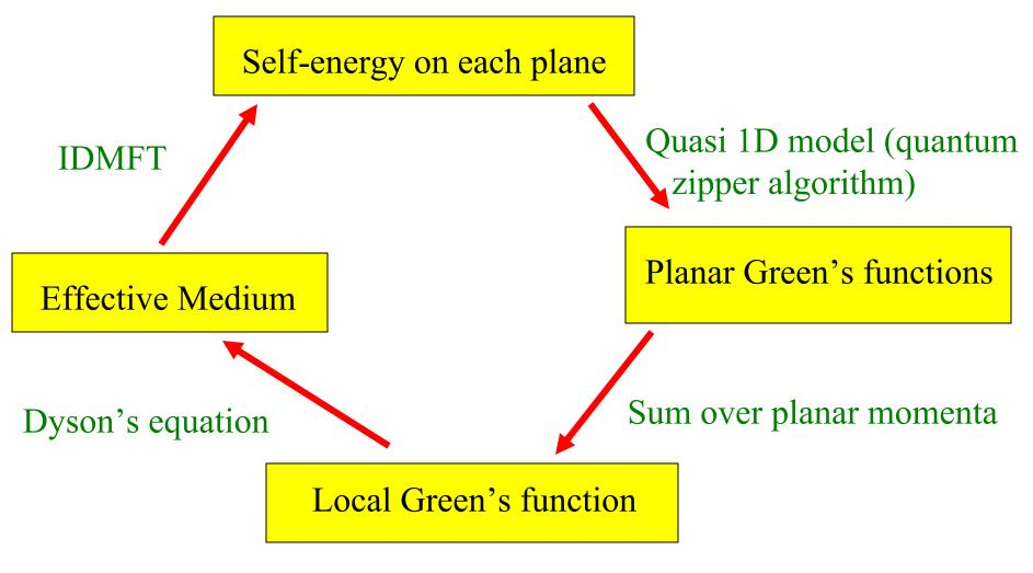
Algorithm is iterated until a self-consistent solution is achieved
