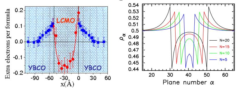
Using a scanning transmission electron microscope with electron energy-loss spectroscopy, one can directly measure the electronic charge at each plane of a strongly correlated multilayered nanostructure. Left are experimental results by Varela et al. on YBCO/LCMO heterostructures, right is a simple theory for a correlated nanostructure.
