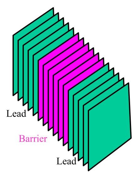
The metallic leads can be ballistic normal metals, mean-field theory ferromagnets, or BCS superconductors.
