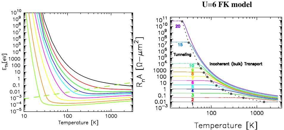
The Thouless energy determines the transition from tunneling to incoherent transport as a function of temperature!
