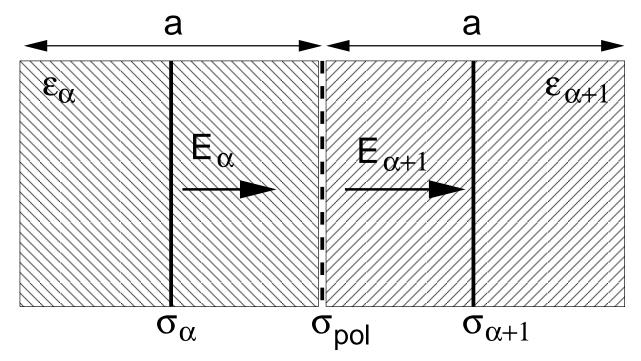
We employ a semiclassical treatment to handle the electronic charge reconstruction. We allow charge to be rearranged on different planes, as determined by the electrochemical potential at a given plane site, and then determine the classical Coulomb potential from planes of net charge, with dielectric constants that can vary from plane to plane.
