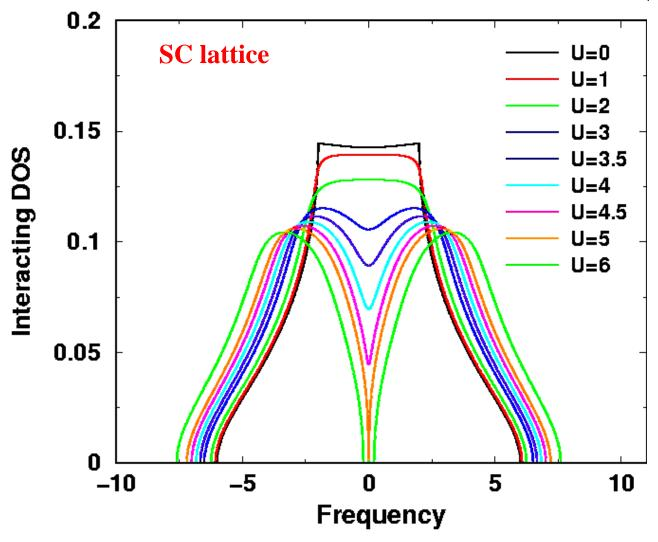
The Falicov-Kimball model has a **metal**insulator transition that occurs as the correlation energy U is increased. The bulk interacting DOS shows that a **pseudogap** phase first develops followed by the opening of a true gap above U=4.9 (in the bulk).
