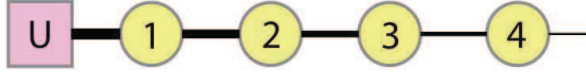
Fig. 5. (Color online) The Wilson chain is constructed similar to a Lanczos procedure, where the impurity is coupled to a linear combination of bath sites, which we denote as the first chain site. The chain site is then coupled in turn to new chain sites, with the coupling between chains decreasing down the chain (indicated by the shrinking widths of the lines denoting the hopping).
