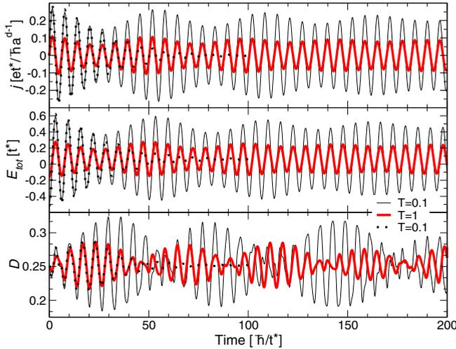
FIG. 7. (Color online) Nonequilibrium (a) current density, (b) total energy, and (c) double occupancy versus time for different values of  $T_0$  with  $E = 1$ ,  $U = 0.25$ . Solid black lines correspond to the SOPT with  $T_0 = 0.1$ , solid bold red lines correspond to the SOPT with  $T_0 = 1$ , and dotted lines to the IPT calculation with  $T_0 = 0.1$ .
