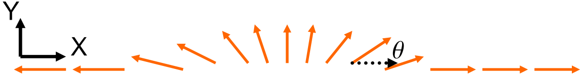
Figure 6. Spin-polarized current enters a half-infinite magnet from the left. Originally the magnetization is aligned along the easy-axis (-x). However if the incoming electrons are spin-polarized in a different direction, their interaction with the magnetization leads to a change of the direction of the local magnetization.
