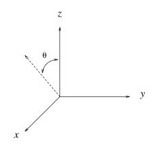
The projection of the needle on the vertical axis is called  $m_z$ . The projection of the needle on the horizontal axis is called  $m_x$ . The projection of the needle on an axis tilted at an angle  $\theta$  to the vertical axis is called  $m_{\theta}$ . Using this terminology, we have  $m_0 = m_z$ ,  $m_{90} = m_x$ , and  $m_{180} = m_{-z}$ .
