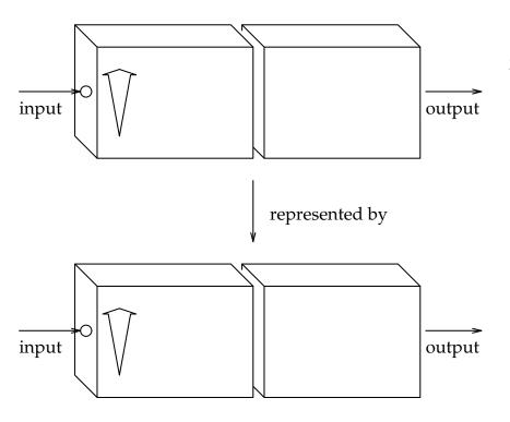
1st box = Stern-Gerlach analyzer 2nd box recombines the paths of atoms leaving the + and - exits.
