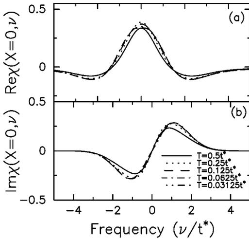
FIG. 8. Dynamical local charge-density-wave susceptibility as a function of temperature for the case  $U=1$ . The real part is plotted in (a) and the imaginary part in (b). Five different temperatures are shown:  $T=0.5$  (solid line),  $T=0.25$  (dotted line),  $T=0.125$  (dashed line),  $T=0.0625$  (chain-dotted line), and  $T=0.03125$  (chain-double-dotted line). We once again see a similarity with the chessboard phase, but the temperature dependence is much reduced here.
