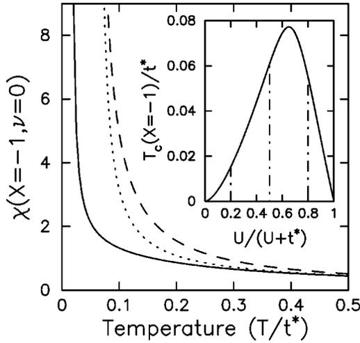
FIG. 4. Static charge susceptibility for the chessboard charge-density-wave plotted versus temperature for three values of  $U$ : (i)  $U=0.25$ , solid line,  $T_c=0.0153$ ; (ii)  $U=1$ , dashed line,  $T_c=0.0608$ ; and (iii)  $U=4$ , dotted line,  $T_c=0.0547$ . The inset is the charge-density-wave transition temperature plotted as a function of the interaction strength  $U/(U+t^*)$ .
