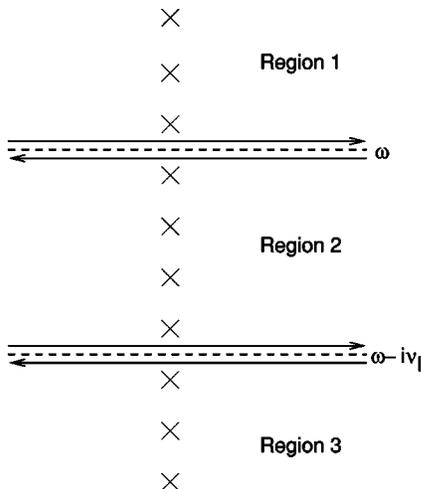
FIG. 2. Deformation of the contours needed for evaluation of the susceptibility on the real axis. The integrations are parallel to the real axis.
