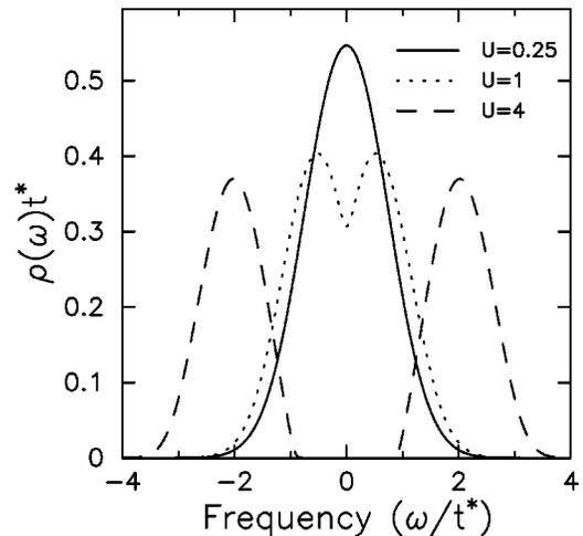
FIG. 3. Interacting density of states for the spinless Falicov-Kimball model at half filling and  $U=0.25$  (solid line),  $U=1$  (dotted line),  $U=4$  (dashed line). Note how the density of states evolves from being essentially Gaussian to developing a pseudogap and then a real gap as the interaction strength is increased. The density of states is temperature independent for this model.
